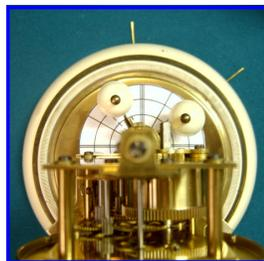
*cates the pin-to-pendulum-ball relation at the end of the pendulum’s swing in the “CCW” direction (showing the “over-swing”). Pins show the precise positions, while the positions using the protractor must be remembered!]*
